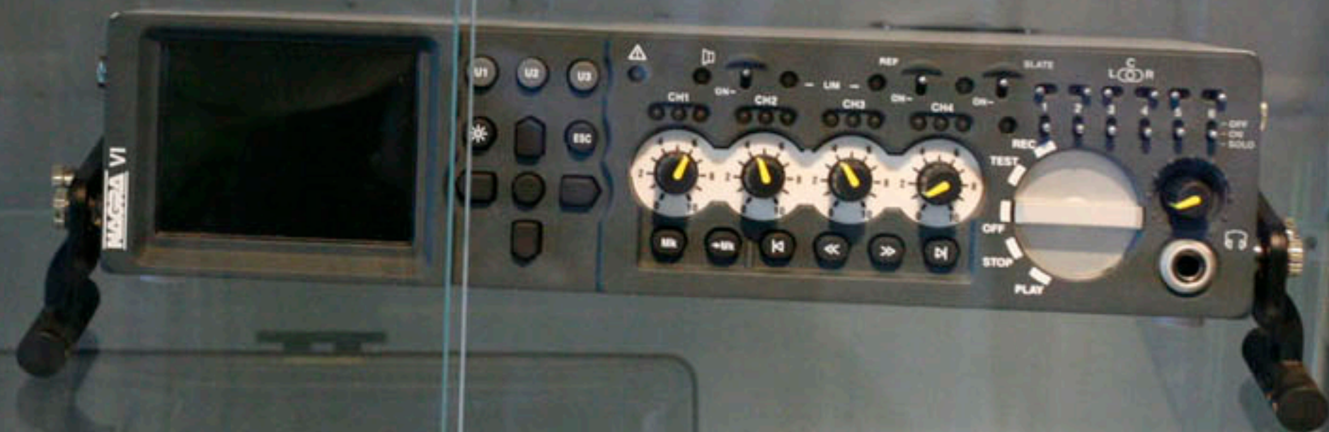
NAGRA NAGRA VI (2008 - ) 6-channel digital recorder using both internal hard disk and removable compact flash media. Includes a built-in mixer and full TC system. Designed for both music and film/TV applications.
