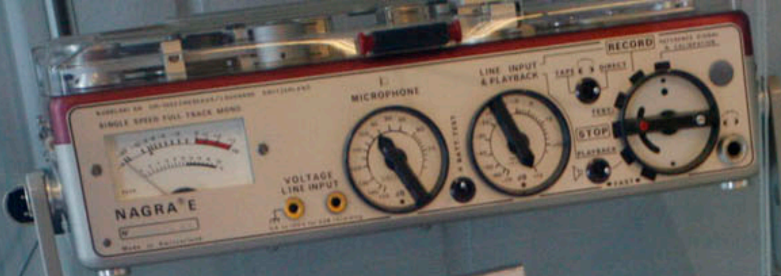
NAGRA NAGRA E (1982 - 2004) Analog "Economic" recorder for in-the-field broadcast, single microphone input and single tape speed.
