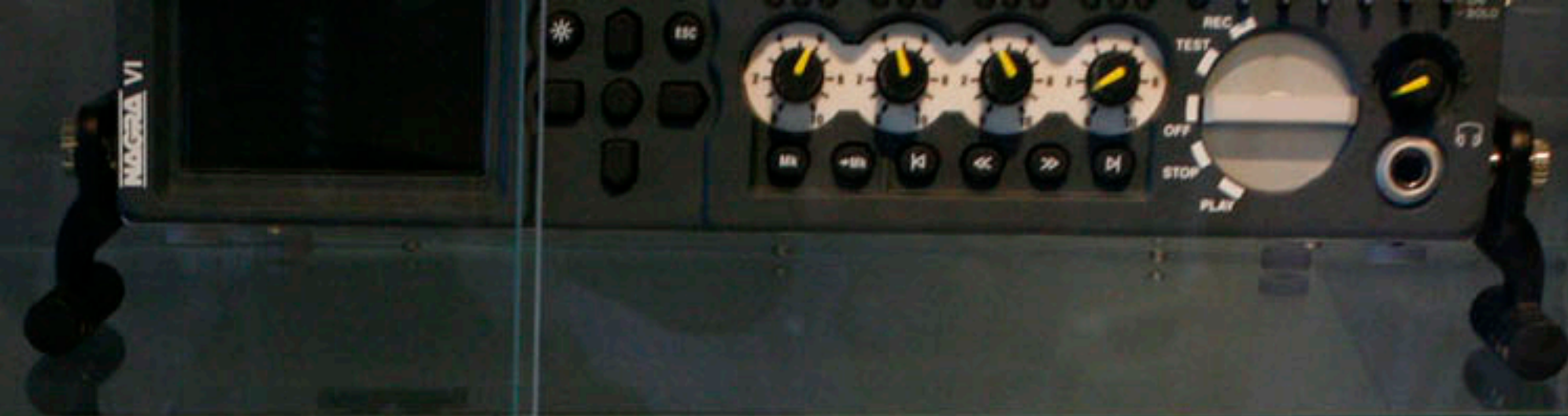
NAGRA NAGRA VI (2008 - ) 6-channel digital recorder using both internal hard disk and removable compact flash media. Includes a built-in mixer and full TC system. Designed for both music and film/TV applications.
