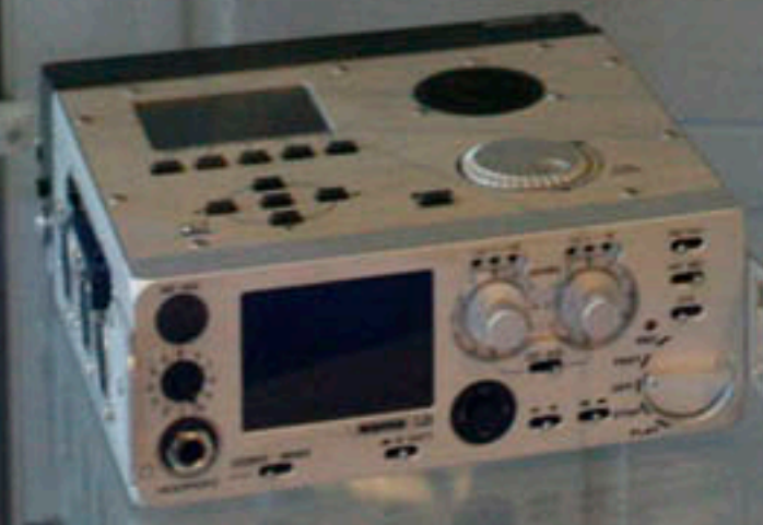
NAGRA ARES-M BOX200 The first non-linear digital recorder to broadcast equipped with on-board editor and VCR modes.
