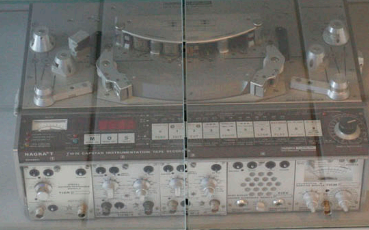
NAGRA NAGRA IV-SJ (1972 - 1991) Analog recorder for instrumentation recording of tone and vibration.
